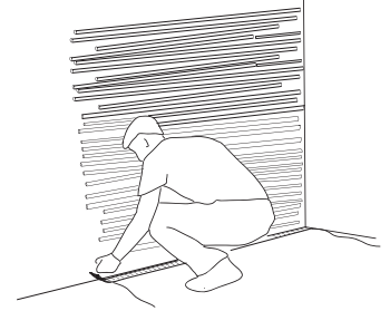
Applying protection for flooring
